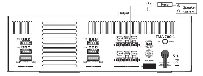
Use the following formula to determine the fuse capacity according to the speaker's input capacity.
